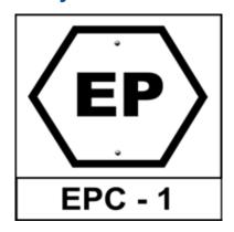
This sign marks the location of the boundary between two TBTC loops. Trains re—entering the TBTC signalling system must ensure that their Vehicle on Board Controllers (VOBC) are reset before passing this sign.
