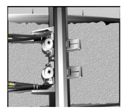
Detects the passing of a train using a counting head (detection point) installed at each end of a section. As each axle passes the head at the start of the section, a counter counts in the axle. A detection point comprises of two independent sensors; therefore the device can detect the direction of a train by the order in which the sensors are passed. When the train passes a similar counting head at the end of the section, the axles are counted out.
