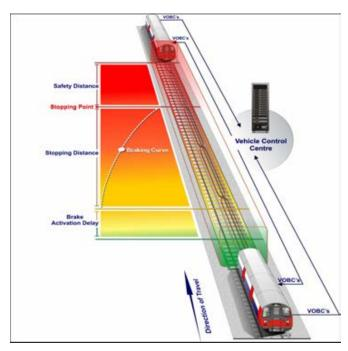
TBTC is a computer based signalling system that is different to the normal conventional system as it does not have:
