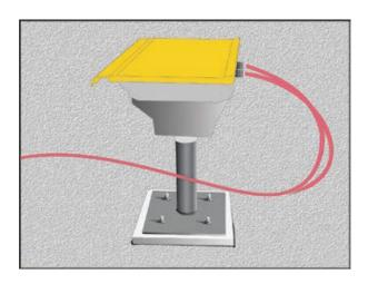
The inductive loops are fitted to the remote loop box via a feed in device that transmits information back to the VCC.
