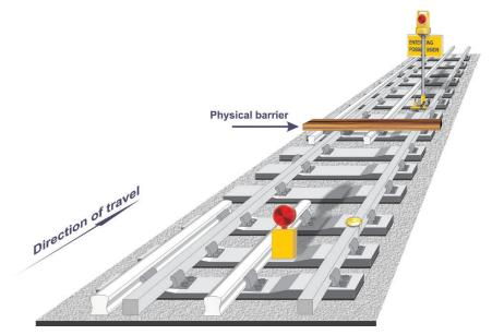
This method of protection can be used in fully un-signalled depots or on un-signalled tracks in other depots. A physical barrier, such as a timber baulk, is placed in the four foot as a warning to train operators that the section of the track concerned is under possession.
