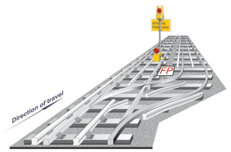
Facing points can be secured, using the approved method, so as to divert trains away from the section under possession. The points must be secured in the normal position unless the points are controlled from one of the signal boxes listed below, when they can be secured in either the normal or reverse positions.
