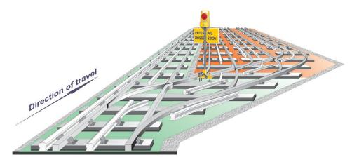
This method of protecting a possession must only be used during Engineering Hours for a minor possession and relies on the Line Clear and Line Safe procedures to provide a protecting 'buffer' traction current section, where traction current is switched off, to prevent unauthorised trains from reaching the traction current section(s), depot or siding under possession.
