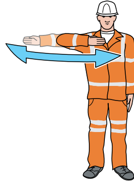
Move towards the shunter
