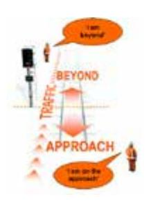
An example is given here, however the terms are used for points or another fixed structure e.g. bridge, gantry.
